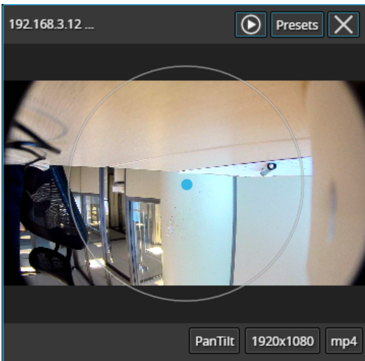
Live view with overlay PTZ controls
