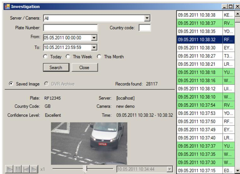
Investigation window is used to examine and search through recognition data. Upper-left part contains search-related options and lower-left part displays a snapshot of recognized plate, if you have enabled snapshot storage or have a DVR archive for the camera where plate was found for the given time.
