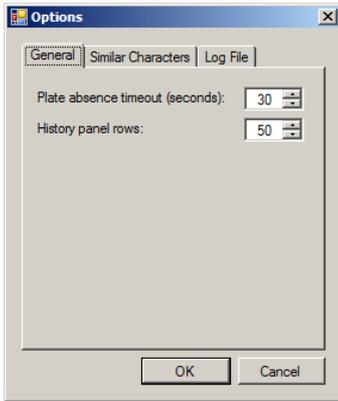
General options. Plate absence time, given in seconds, defines how long licence plate should be out of view to get recognized again. This is useful, for example, if parked cars might appear inside recognition area. A person walking by and covering plate for few seconds will not trigger re-recognition.
