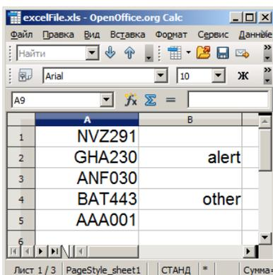
This is example contents of an MS Excel file. First column contains triggering number plates. Second, optional column, contains additional information about number plate, which is referred to as a Triggered Plate Tag and can be supplied as command-line argument, **TriggeredPlateTag**. You can check what number plates are currently triggering under *Tools -> Trigger Plates* menu
